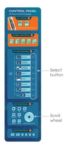
Run the stylus tip of your FLY Fusion Pentop Computer around the scroll wheel (•) to scroll through your songs.
